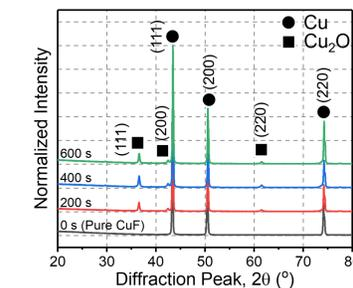
Figure 7: Normalized XRD pattern.
