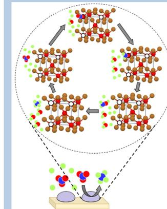
Figure 11: NO<sub>x</sub>RR reaction mechanism by Cu<sub>2</sub>O.
