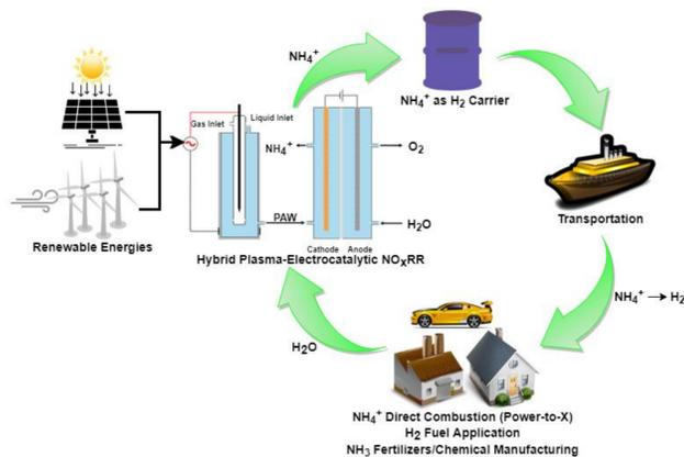
Figure 3: Complete green NH<sub>3</sub>/NH<sub>4</sub><sup>+</sup> production.
