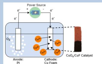
Figure 4: Electrodeposition process.
