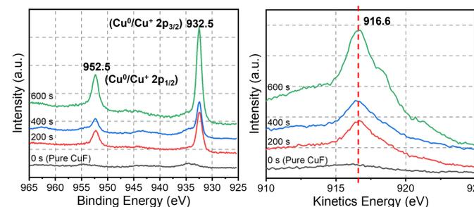
Figure 8: XPS spectra of (a) Cu 2p and (b) Cu LMM.
